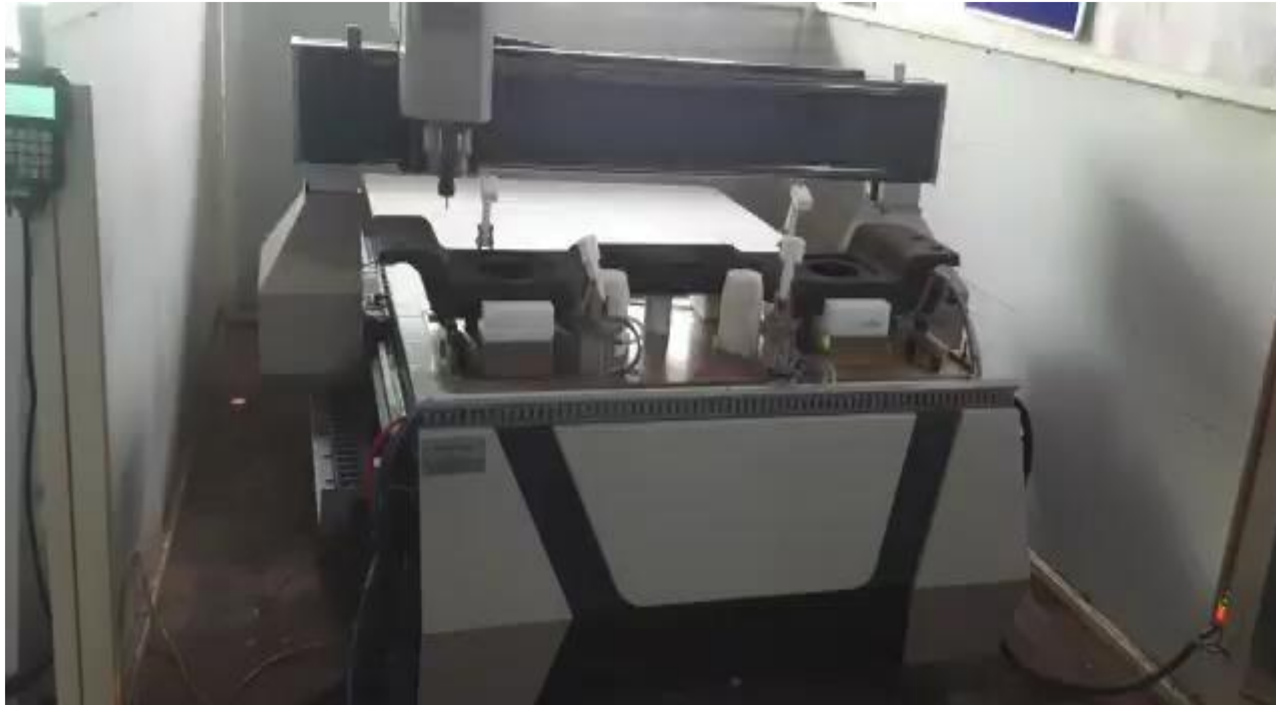
CNC Router with fixture for speaker trimming in plastic part – Minda Group, Bangalore
