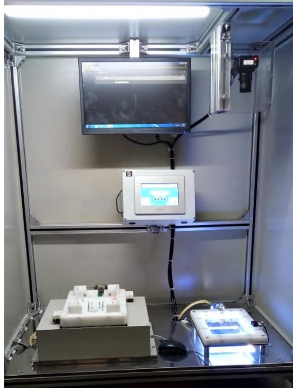
Flash in mould inspection with camera Sumi- Motherson Pondicherry
