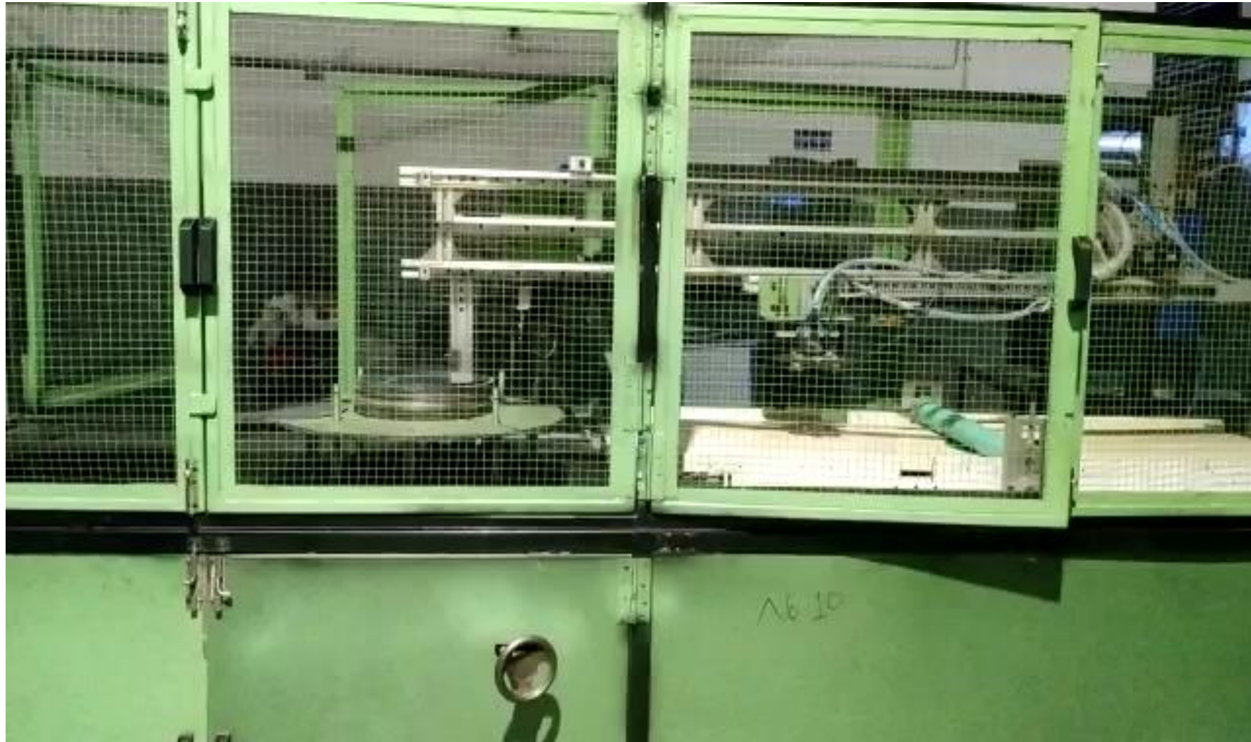
Man less Loading & Unloading with coolant applicator. Milton, Haridwar
